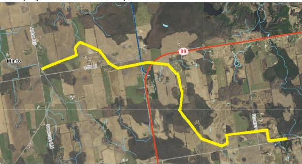
During investigations and conversations with property owners at the south end of the drain near the 12<sup>th</sup> Line it was determined that to get the necessary fall to accept their private field tile systems, work may be required in sections all the way to the outlet. The Town received three separate signed section 78 request for upgrades to the entire system.
