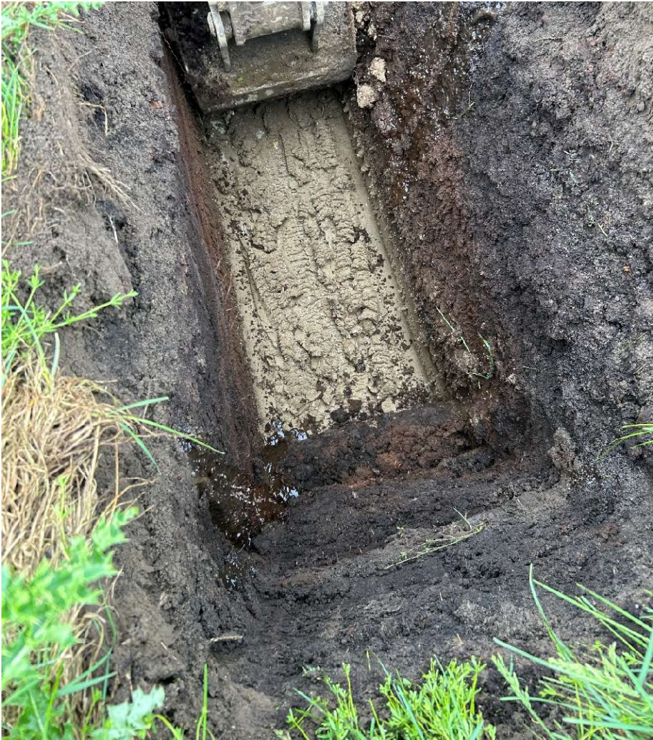
Figure 1 – Unstable soil with high organic content within the low-lying lands on Lot 7, Concession 8
