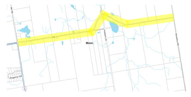
3) Sand pad and resurface the Blind Line and the 8<sup>th</sup> Line to at least Road 3 N and possibly to Pike Lake Sideroad (this has not been in the Town 5 year plan but based on the increased traffic flows from Minto Ag and increased Mennonite Businesses it has deteriorated faster than anticipated)
