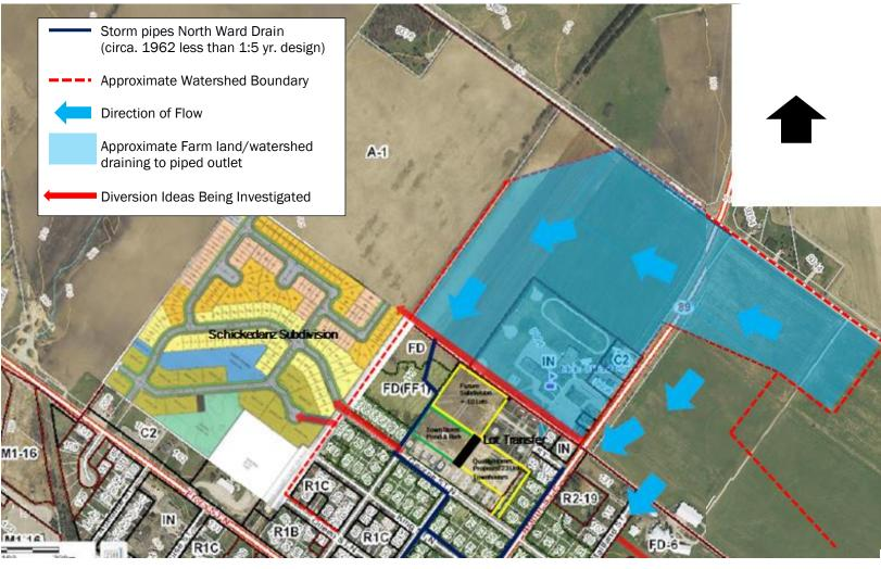
At least 60 acres of land drains to the top end North Ward Drain inlet located west of William Street. Over 14 more acres drain into another arm of the North Ward Drain at the end of Maitland Street. Direction of flow is shown on the map above with the large blue arrows. The black strip on the map (Land Transfer) represents the less than 0.29 acres to be sold to
