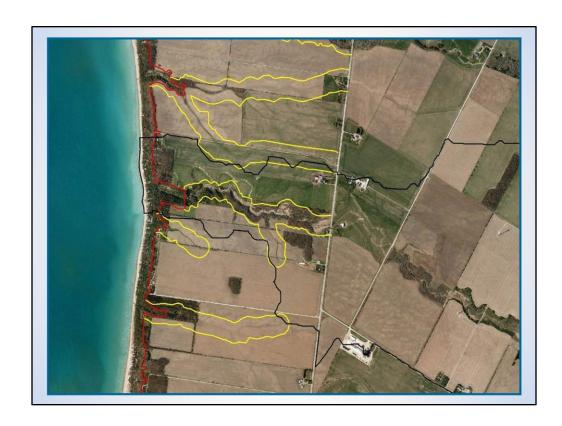
This slide illustrates the land that is and will be affected by gully erosion if no storm water management system is put in place. Red lines show development at risk from shoreline/bluff collapse.
